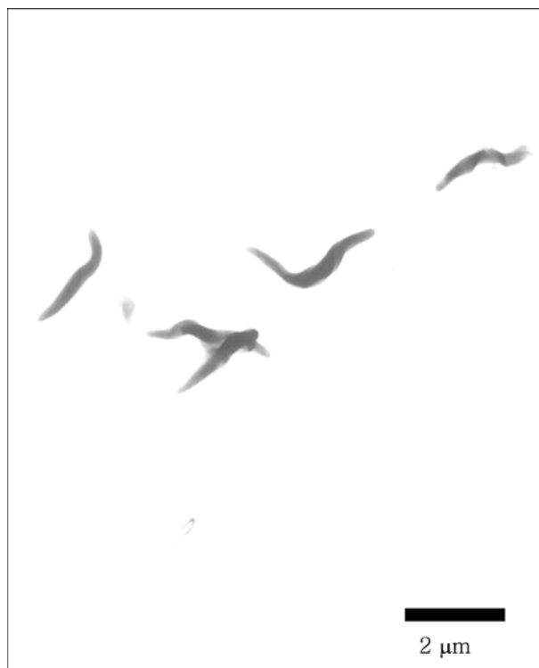
Fig. 3 TEM image of precipitated PANI particles
